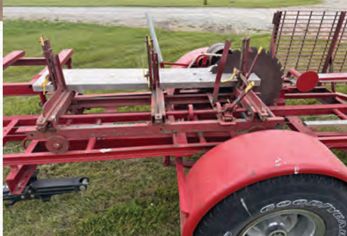
LOT #390 1/2 SCALE PORTABLE SAWMILL EXCELLENT running sawmill. 20" blade cuts 8" log 6' long. Works well on the 1/2 scale steam engine or one of the 8 HP Hit N Miss engines.
